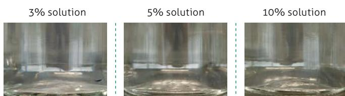
**LUBARIT® EXP 6533/1** dissolves completely in DI water and is perfectly stable at all dilution rates.
