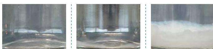
**COMPETITOR B** Compatible and stable at low treat rates. High treat rate results in solid flocculation.
